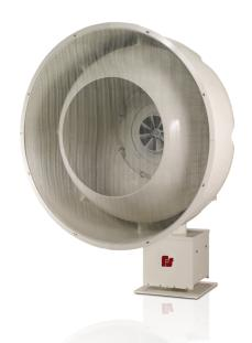
Federal Signal's 508-128 siren is a high power, rotating, unidirectional, 500 Hz outdoor warning siren that offers an anechoic chamber-certified of 128 dBc. The high-decibel output provides maximum coverage with minimum installation cost. Radio activation can further minimize installation costs by eliminating the need for leased dedicated control lines.
